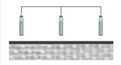
In this working mode all the sensors measure simultaneously. All sync terminals (SYNC) must be connected to each other and the system must be powered.
