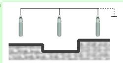
In this working mode the sensors measure in a chain. All sync terminals (SYNC) must be connected to each other and also to ground (Vss). Power up the system and after 5 seconds disconnect SYNC from the ground.
